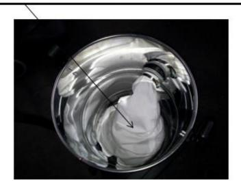
To remove the bag, the operator must disassemble the iron band
